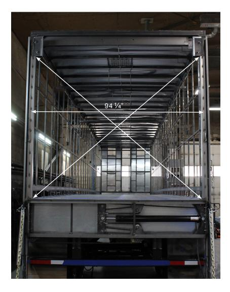
Step 11: Install <sup>3</sup>/<sub>8</sub>" hydraulic hose(s) to cylinder. You should now be able to activate cylinder and raise the 5' slider tubes 18" off the ground. You are now ready to install the platform to the slider tubes using the 1 <sup>1</sup>/<sub>2</sub>" steel platform pins and lock collars. Fold platform into an upwards position and install <sup>3</sup>/<sub>8</sub>" chain with quick link to 5' slider. Also, spring balance assembly to slider and platform.
