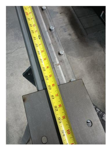
Step 8: Attach left and right chain to 5' sliders. Grease sliders and insert into left and right 10' rails, pulling the chain up as you go. Thread chain around top sprockets and clamp roller chain to 10' tubes. To ensure that they are in the correct tube, the cutout in the slider will be on the same side as the two roller sprockets in the top of the 10' rails. Install bottom sprockets in the 10' rails and thread chain as shown.
