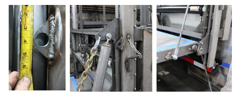
Step 14: Weld bottom cylinder box supports in place. See picture. Weld cylinder box and 10' rails securely to the back of the trailer. Install safety chain to secure platform in traveling position. This will be approximately 16" up from trailer floor and hook into the 3/8" platform chain.
