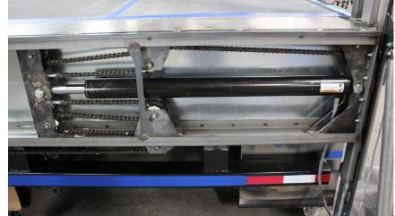
Step 12: Raise platform to floor height of trailer. Use chain adjusting bolts to level platform with floor. Begin greasing 10' rails with lithium grease. Now, you want to weld the platform latch. Position the bottom of platform latch approximately 31" up front floor and weld into place. See picture.
